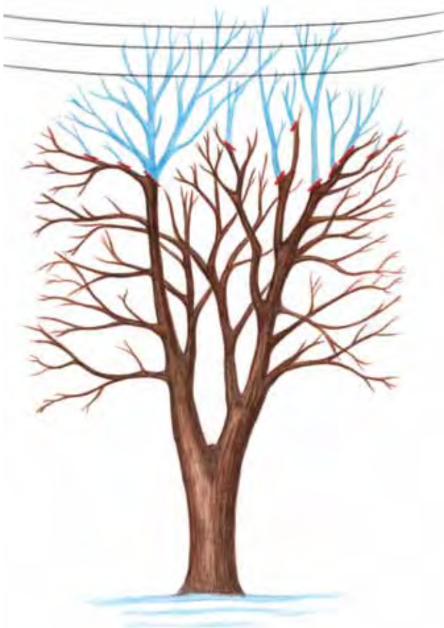
Figure 5. Crown reduction—branches to be removed are shaded in blue; pruning cuts should be made where indicated with red lines. To prevent branch dieback, cuts should be made at lateral branches that are at least one-third the diameter of the stem at their union.
