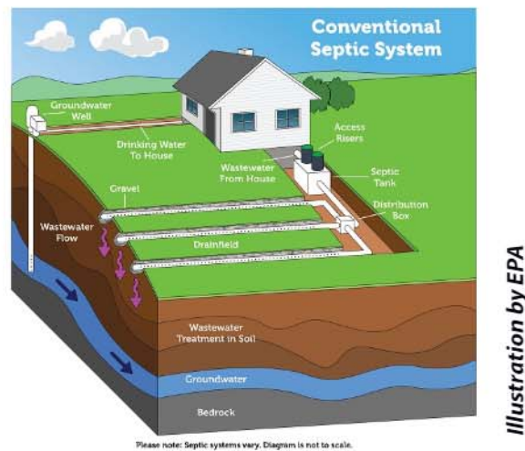
Figure 1: Typical composition of an on-site wastewater treatment system.
